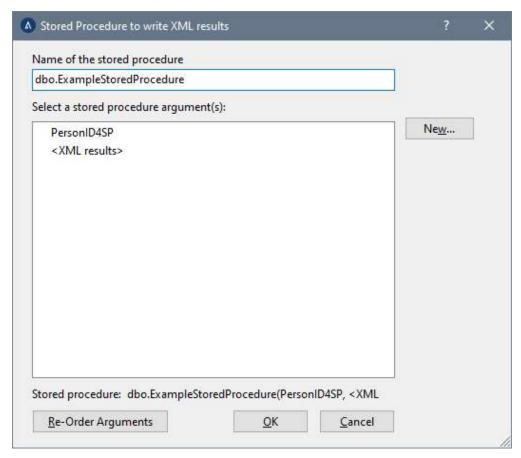
Stored procedure arguments will be listed for review and editing. The required default argument <*XML results*> will pass the calculation results to the SQL database in XML format. You may add any other arguments needed to uniquely identify the calculation and satisfy any Key requirements of the table you are updating with calculation results. Additionally, you can reorder your arguments to align with the stored procedure's expectations.
